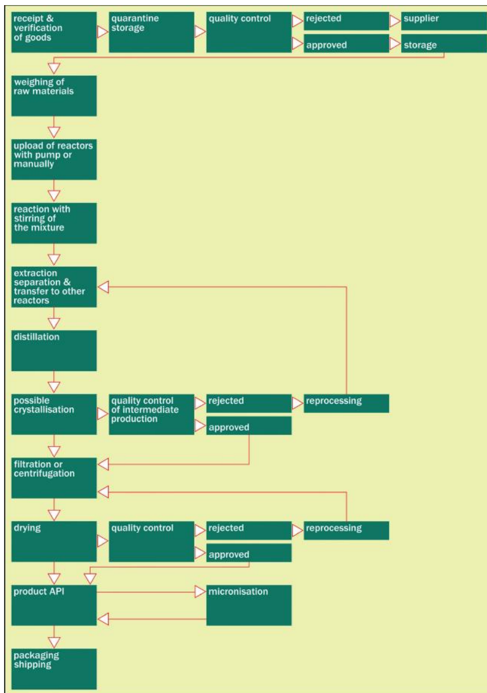
Figure 3.3: Overview of the production cycle, including micronisation stage
